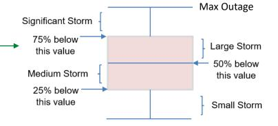
Threshold "Y" is calculated based on data analytics of small, medium, large, and significant size storm with 5 year moving average data. Details are explained in IEEE distribution resiliency guide.
